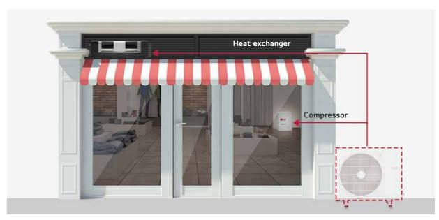
Heat exchanger module can be installed in false ceiling spaces
